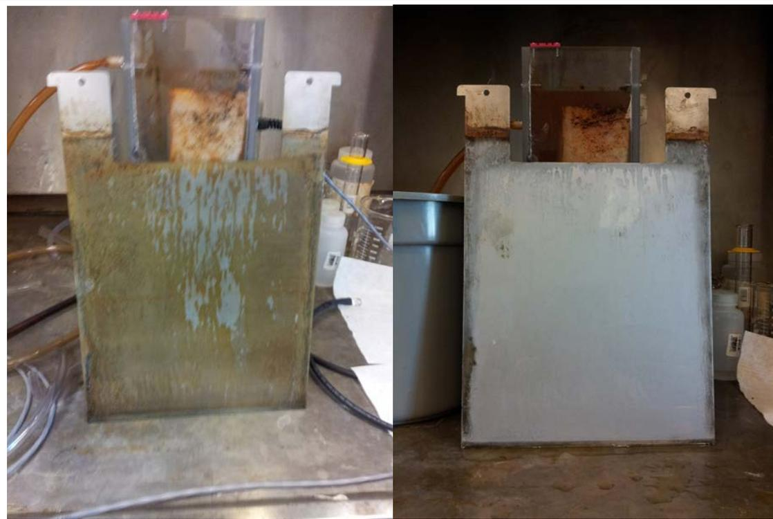
**Figure 2. On the left - “fouled” electrode; on the right - plate after 2 min of ultrasound treatment**
