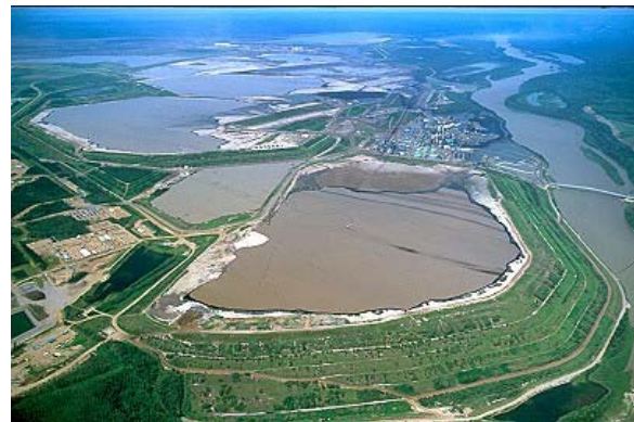
Figure 10.1 – Existing Oil sands Tailings Ponds Located Adjacent to and Above the Athabasca River (left side of photo)
