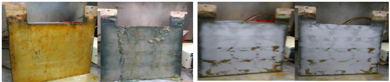
Figure 3a Fouled cathode (left) and anode (right) Figure 3b Defouled anode 2 minutes (left) and 4 minutes (right)
