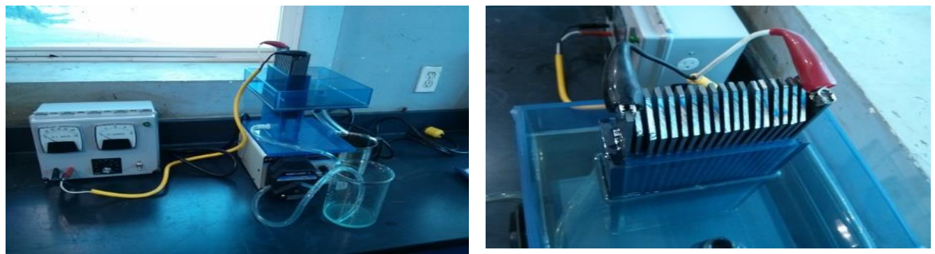
Figure 2a. EC unit for Total hardness Analysis (Left) Figure 2b. Electrodes inside test chamber (Right)
