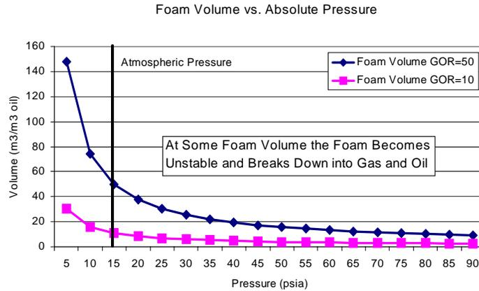
**Figure 5.3 – Heavy Oil and Gas Foam Volume vs. Pressure
