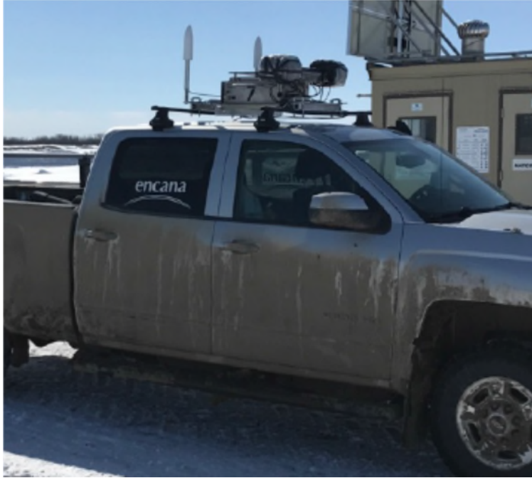
Figures 1 and 2. Sensors mounted on the roof of Encana's vehicles
