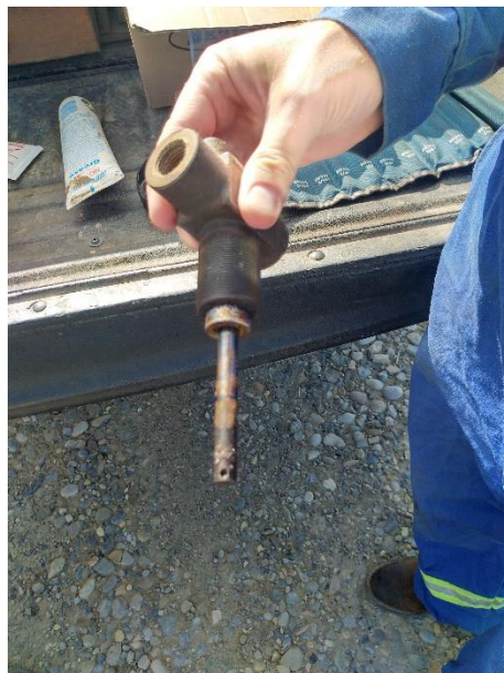
Picture 2. Photo of a 3/8" plunger head of a Bruin 5100 pump, which was replaced with a 1/2" plunger.
