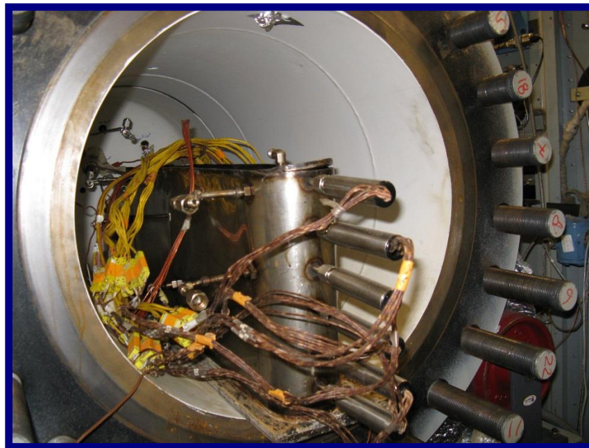
Figure 8-4. Scaled physical model for thermal oil recovery process experiments.
