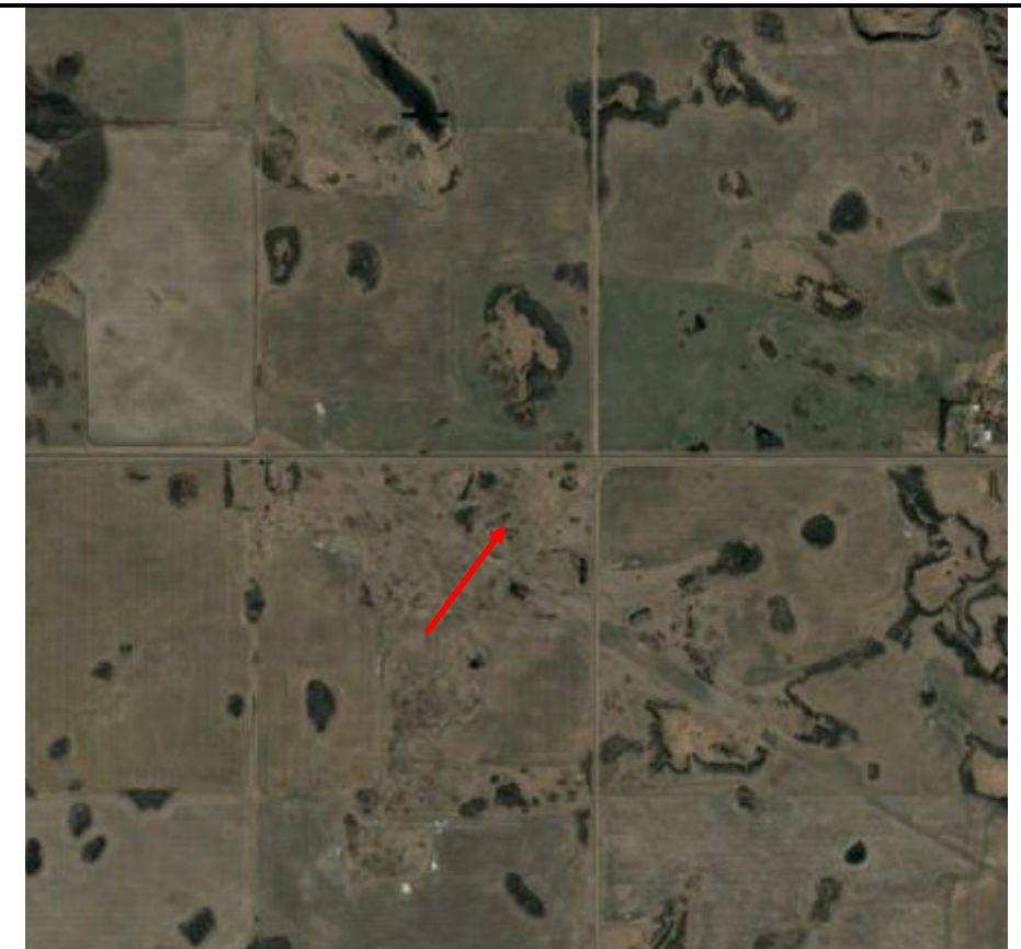
Photoplate: Aerial view of temporary marsh area (Google Earth, September 29, 2018). There is evidence of the formation of additional wetlands adjacent to the pipeline corridor that may represent preferential drainage along the outside of a pipeline. However, given that the abandoned Segment 1B is collocated in a corridor with other active pipelines, the formation of these wetlands cannot be conclusively attributed to Segment 1B. Additionally, there was a significant amount of precipitation (i.e., snow and rain fall) in September 2018, that may have contributed to the accumulation of water in depressions adjacent to the pipeline corridor.
