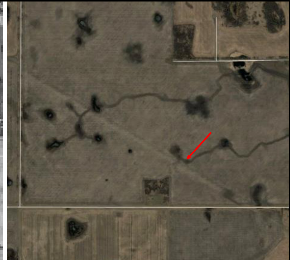
Photo-plate: Aerial view of subsidence area (Google Earth, September 29, 2018). This image was taken approximately 38 years after the abandonment of Segment 1B.
