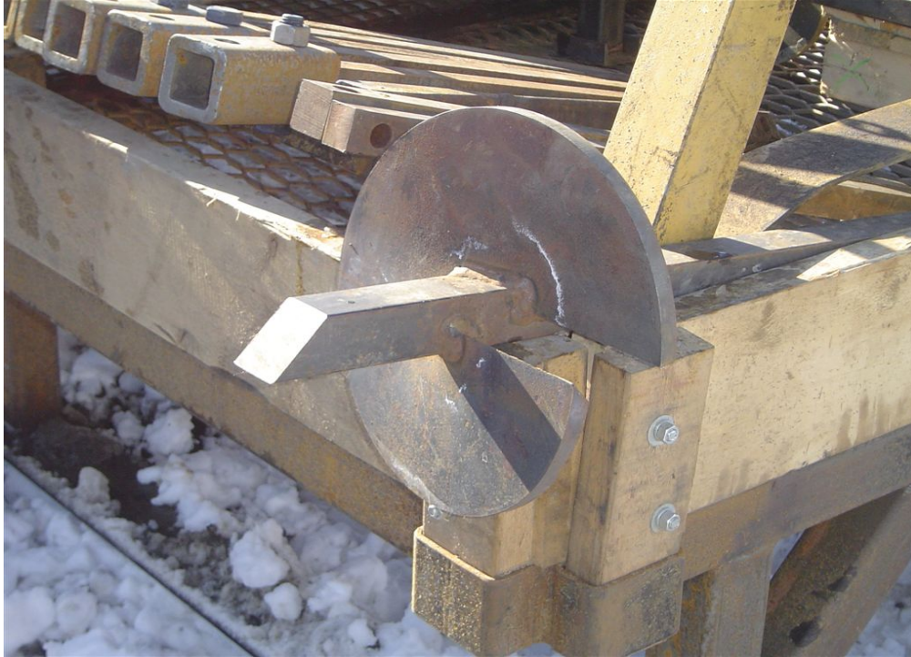
Figure 7 Power Driven Steel Screw Anchor Lead Section (typically only a single helix, see also the connecting bracket at top left; photo courtesy of A. Brown, AHB Consulting)
