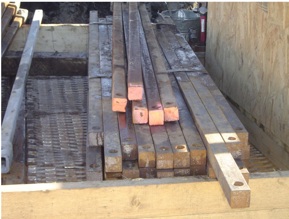
Figure 8 Screw Anchor Extensions (1.8 m long) (photo courtesy of A. Brown, AHB Consulting)
