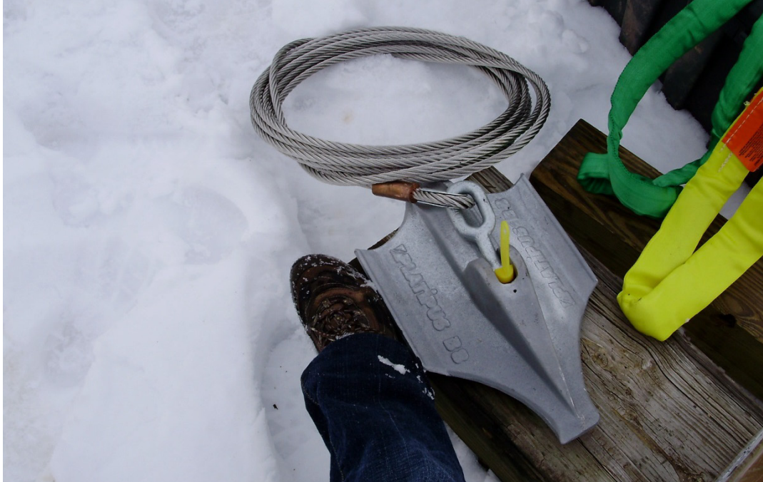
Figure 11 Mechanical “Flip” Anchors & Cable (Platipus anchor: http://www.platipus-anchors.ca ; photo courtesy of J. Keaton, Wood PLC)
