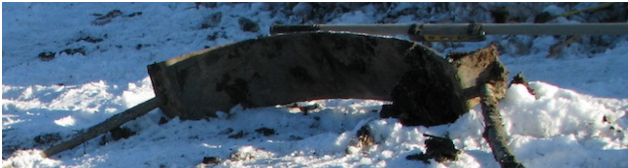
Figure 21 Excavated 40+ Year Old Screw Anchor Saddle in Northeast BC (photo courtesy of A. Brown, AHB Consulting)
