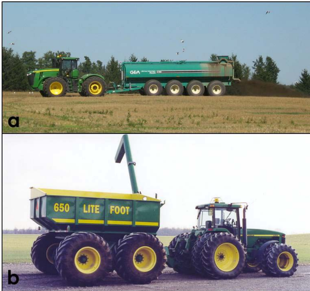
Figure E-5. The level of ground pressure exerted on the soil by modern, often over-sized agricultural equipment, such as a) liquid manure tankers, and b) grain carts, can be diminished with flotation tire systems. (photos: R.A. McBride).
