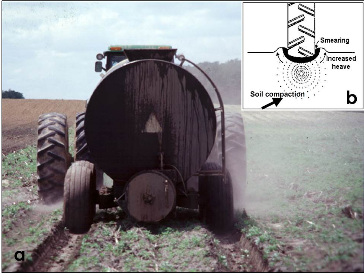
Figure E-6. An illustration of a) high axle-load wheel traffic on an agricultural field near Embro, ON (photo: R.A. McBride), inducing b) deep soil rutting as the soil reacts to forces exerted by the tires of a tractor and a liquid manure tanker.
