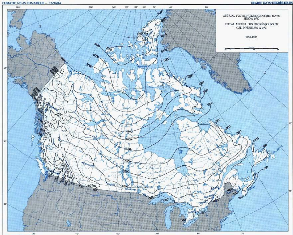
Figure D-5. Map of annual total freezing degree-days below 0°C across Canada. (after Environment Canada, 1988).
