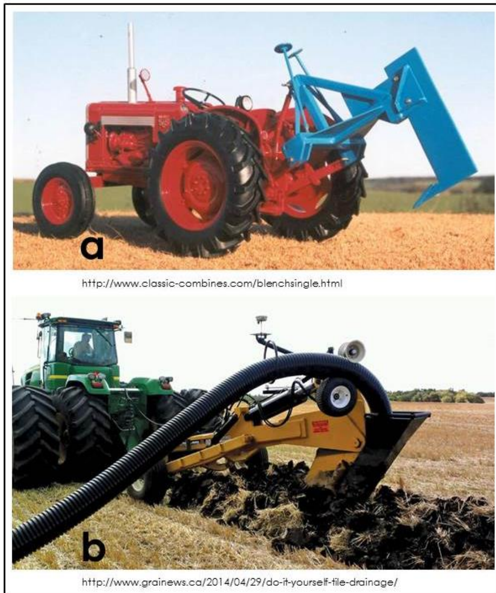
Figure 2.10: Typical farm practices in southern Canada often include a) sub-soiling and deep-ripping operations, and b) sub-surface file drain installation.
