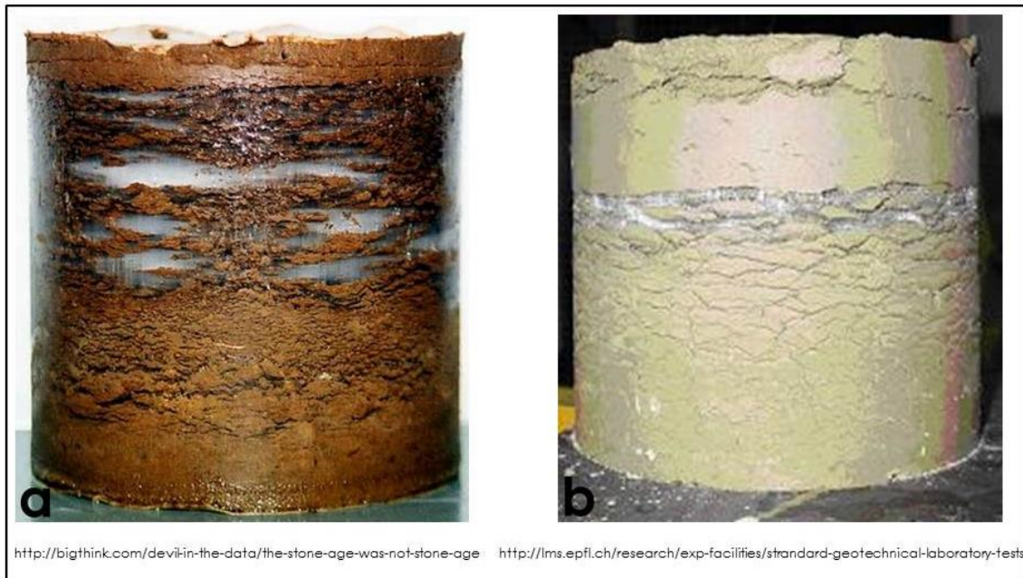
Figure 7.2: Soil columns after laboratory freezing tests, showing wall-to-wall ice lens continuity in soils that are a) well aggregated, and b) structureless (single grain).
