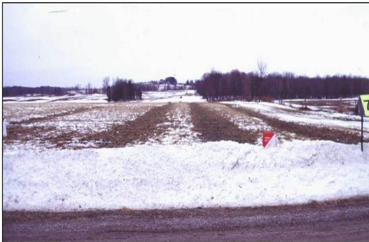
Figure 2.2: Soil heating downstream from a natural gas compressor station in January near Bright, ON (photo: R.A. McBride).
