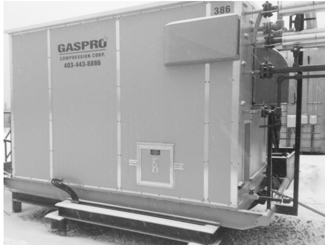
Figure 4 - GasPro BTEX VRU
