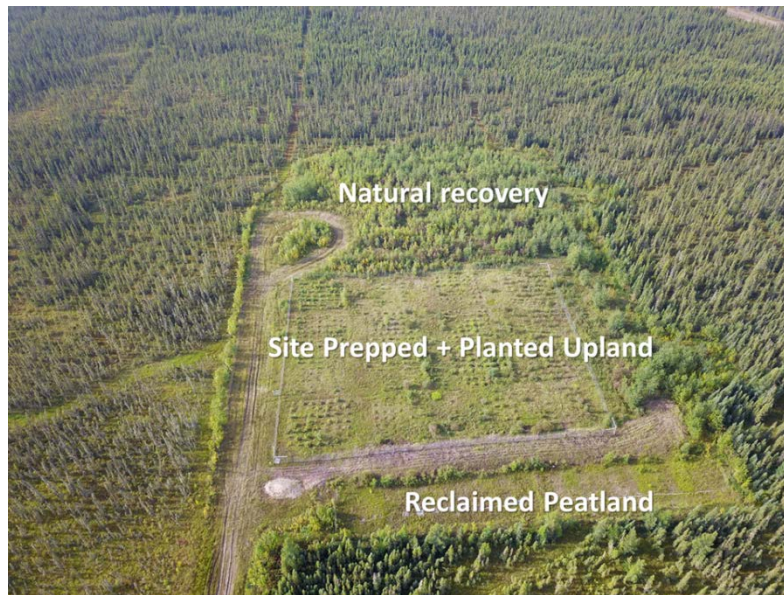
Figure 6. An example of a reclaimed well pad in a peatland. Showing a naturally regenerated section (natural recovery), a fenced section with site preparation (mounding, ripping) and planting of seedlings, and a peatland section reclaimed by partial pad removal and donor fen moss transfer.
